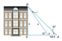
$\Delta DBC$  is a right triangle with hypotenuse of length *a* or about 407.2 feet. You know the measure of the angle at *B*, 55°, so use sine of  $\angle DBC$  to find the height of the building, *h*.
